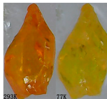
Figure 7. Thermochemical behavior of 1 : Digital photograph of a crystal taken at room temperature (293 K) and temperature of liquid nitrogen (77 K).
